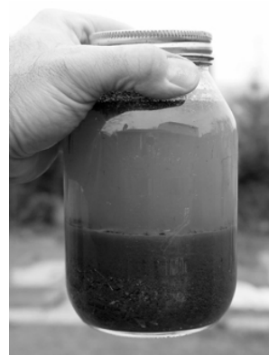
Jar test checks quality of soil
